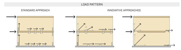
Horizontal loads acting at the floor level introduce shear and tension forces on the structural elements of the building; these forces must be absorbed by an effective connection system. A complete range of joints for walls and buildings also allows for innovative design approaches.
