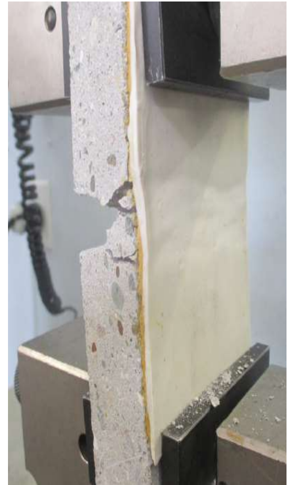
*Elongation of the membrane at substrate crack 6.35mm
