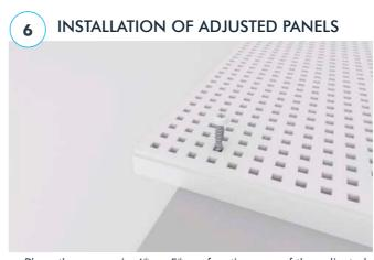
• Place the screws in 4<sup>th</sup> or 5<sup>th</sup> perforation row of the adjusted panel for easier screw-fixing.
