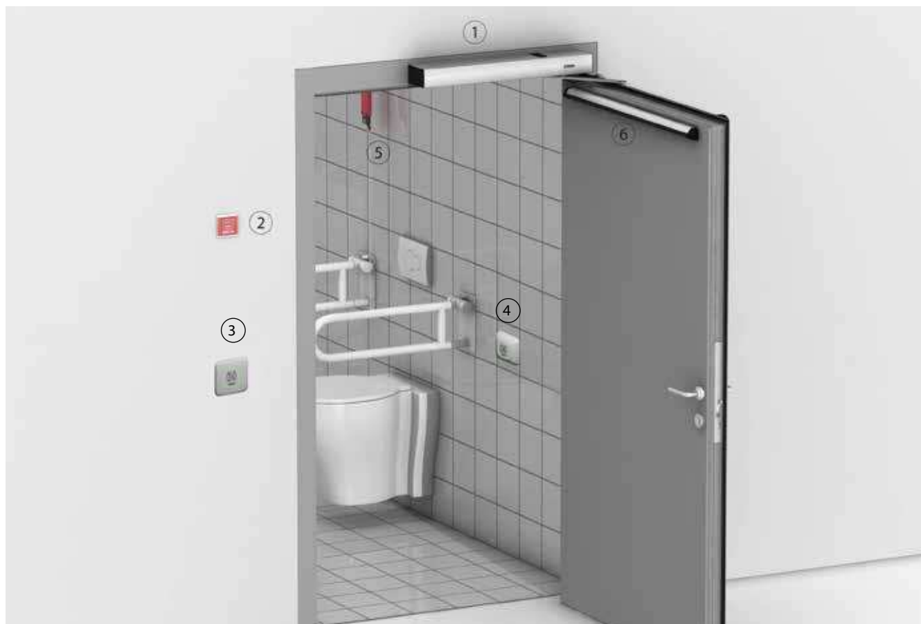
1 = Swing door drive | 2 = Not-Auf Schalter (recommended installation height: 1600 mm) | 3 = Non-contact proximity switch (flush-mounted) | 4 = Non-contact proximity switch (surface-mounted) | 5 = Pull switch emergency call | 6 = Sensor strip
